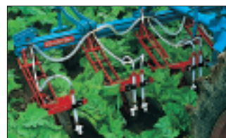
Underleaf spraying in row crops
